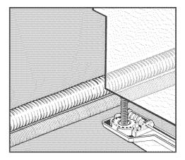
Slide the machine into the opening, making sure the electrical cable and hoses can reach their connection points without kinking.
